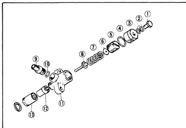
NOTE: Greatest possible care should be taken in handling the nozzles as they are very precisely machined. The nozzle and the needle valve are matched pairs. Do not mix their original combinations. Disassemble and wash each nozzle assembly separately.
