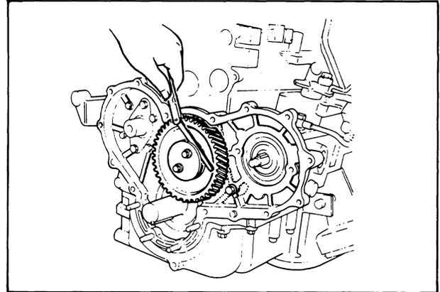
NOTE: Measure the end play after tightening the idler gear attaching nuts to the specified value.
