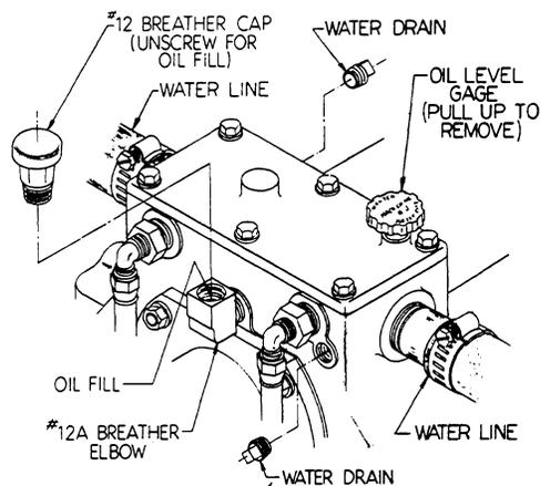
Additional Molykote after break-in is not required. Reinstall the breather cap. The oil level should be rechecked after the unit has been run and allowed to sit for about a minute. Add oil if necessary.
