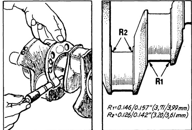
NOTE: Measure the diameter of each of the crankpins and main journals at two points (the front and rear portions) at 90 degrees to the crankshaft axis, as shown in figure.
