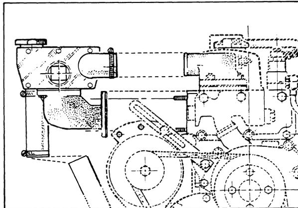
14. Remove the air intake silencer.
