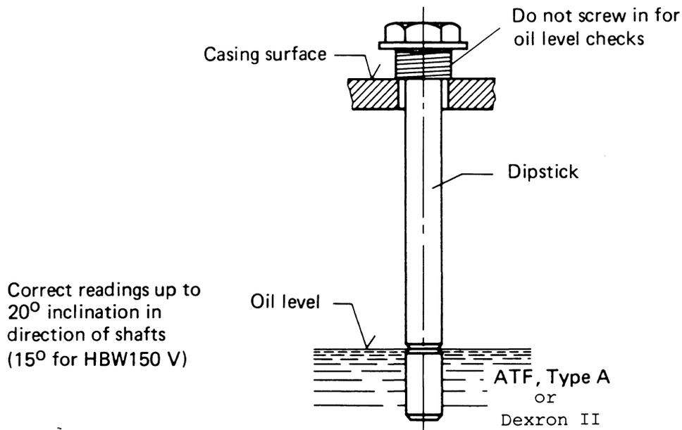
To check the oil level, just insert the dipstick; DO NOT SCREW IN. Retighten the hex screw with the dipstick after the oil level check. Do not omit the o-ring seal.
