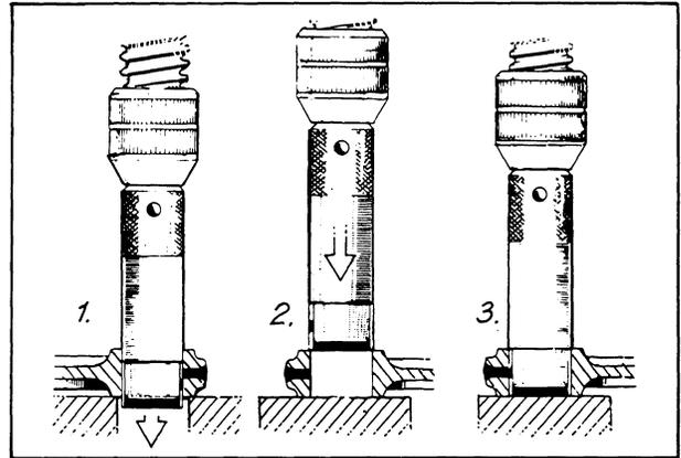
NOTE: When reaming the bushing, correctly insert the reamer in the bushing. In order to prevent unevenness on the bushing surface, the reaming should always be made in the cutting direction. Make sure that the reamer is stopped at different positions at all times.
