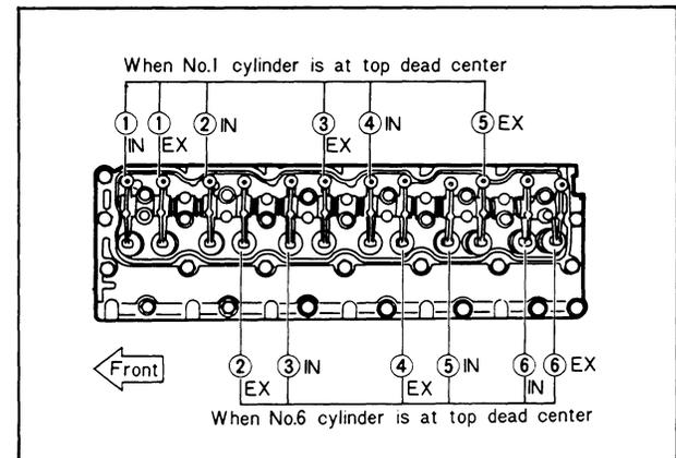
NOTE: When the engine is overhauled, run the engine under load to check its performance. Allow the engine to cool to room temperature and retorque the cylinder head holddown nuts and re-adjust valves.
