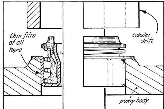
DO NOT ALLOW OIL OR GREASE TO CONTAMINATE THE SURFACES OF THE CERAMIC RING OR THE GRAPHITE (SMALL END) OF THE SPRING-LOADED SEAL.
