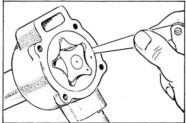
3. Check the end float of the rotors. Place a straight edge across the pump body and measure the clearance between the rotor and straight edge with a feeler gauge. If the clearance exceeds the limit, replace the drive gear, drive shaft, inner rotor, outer rotor and pump body.
