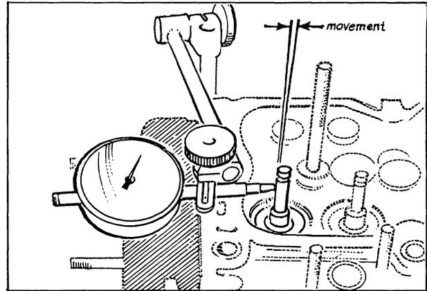
2. Check the protruding length of the valve guide. If it is not the specification, correct it.
