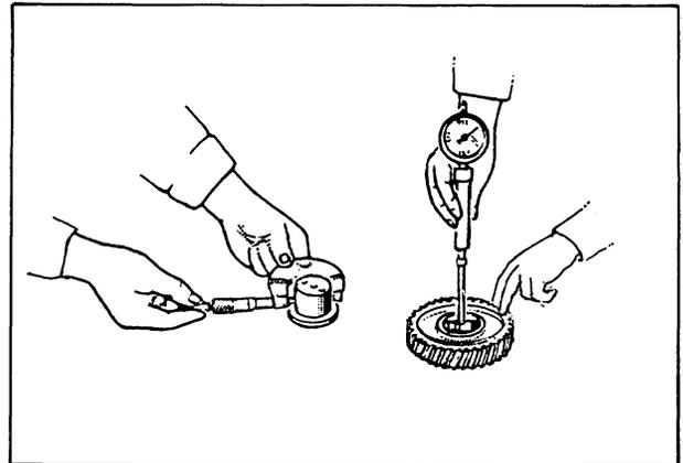
Clearance between bushing and spindle:
