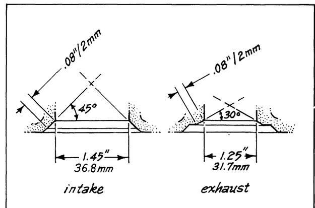
3. Reface the valve and valve seat with a good valve lapping compound.
