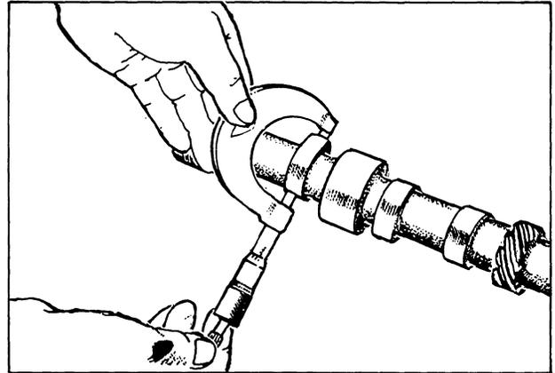
2. Check the cam height and replace the camshaft if the wear exceeds the limit.
