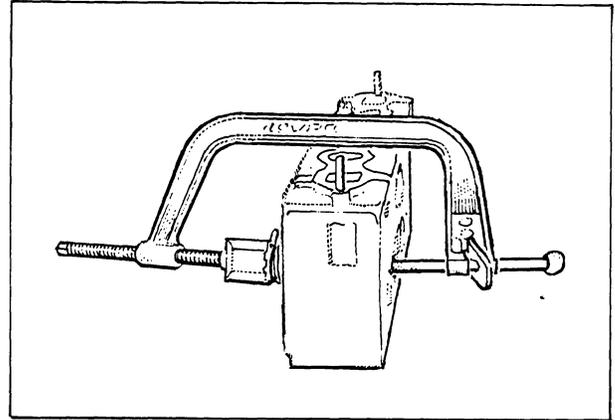
NOTE: After removing the valve assemblies, arrange or label them in the order of removal so that they can be reinstalled in their original positions.
