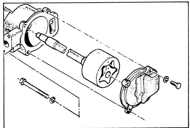
Cover tightening torque: 0.8 - 1.2 kg-m (5.8 - 8.7 lb-ft)
