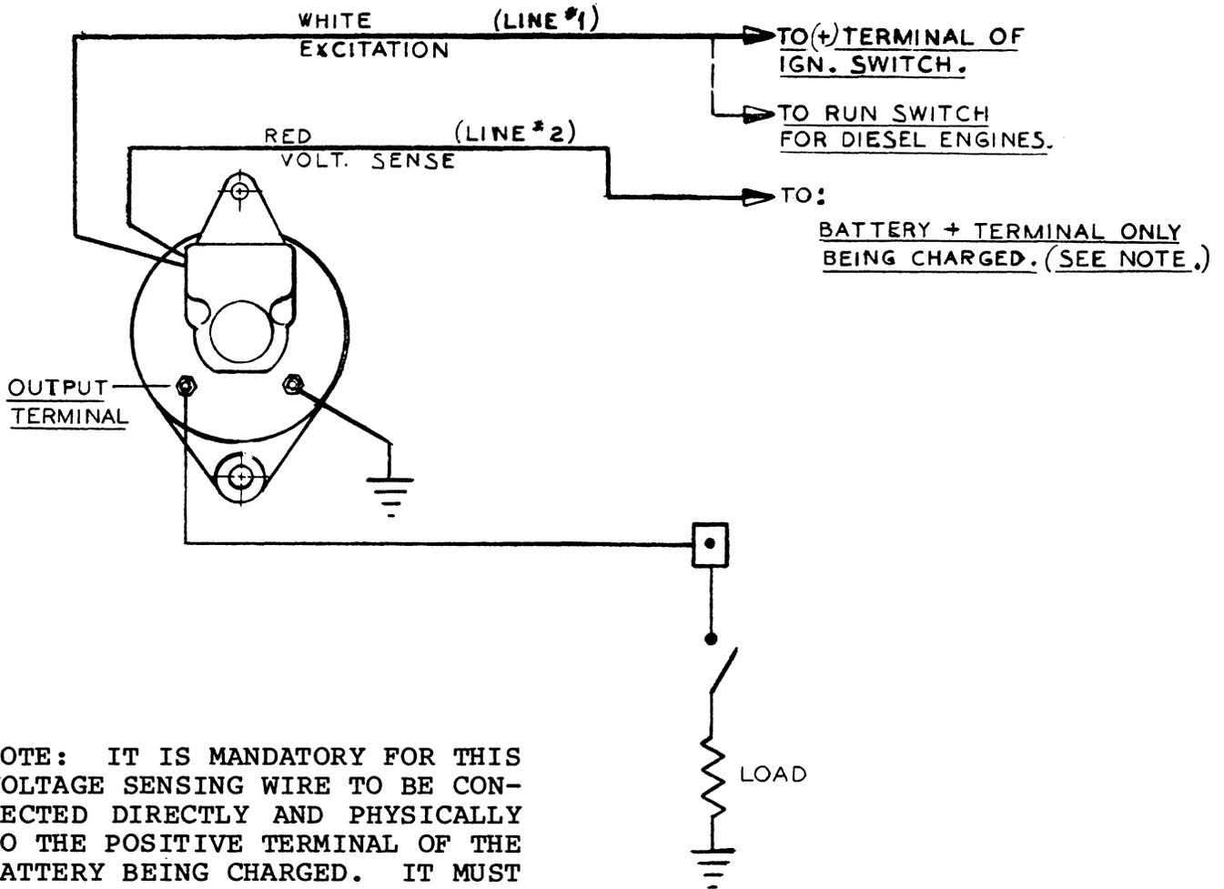
NOTE: IT IS MANDATORY FOR THIS VOLTAGE SENSING WIRE TO BE CONNECTED DIRECTLY AND PHYSICALLY TO THE POSITIVE TERMINAL OF THE BATTERY BEING CHARGED. IT MUST NOT BE CONNECTED TO ANY OTHER CONNECTION POINT. OTHERWISE, THE ALTERNATOR WILL NOT OPERATE PROPERLY.
