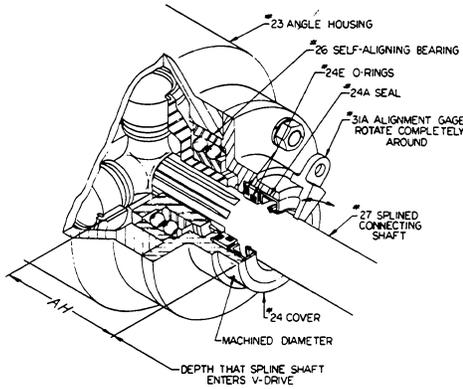
to the joint end that is on the spool adapter. This distance will not vary with misalignment since the joint is bolted and cannot move.) Put the #31A alignment gage on the machined diameter of the #24 cover and slide it completely around. It will indicate how the engine must be moved to center the spline shaft in the oil seal. Re-measure the joints to see if
