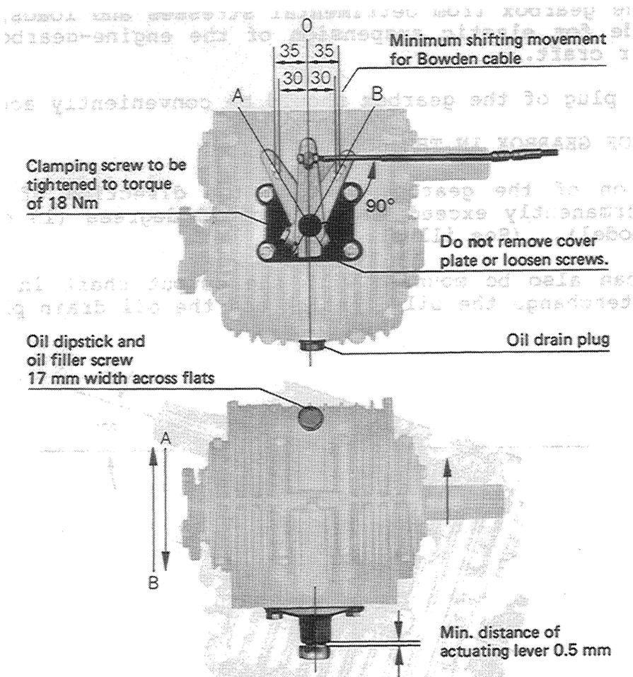
The position of the cover plate underneath the actuating lever is factory-adjusted to ensure equal lever travel from neutral position to A and B. Therefore, do not loosen the capscrews mounting this assembly. Removal or disturbing of the shift cover will void all warranty responsibilities by Westerbeke.
