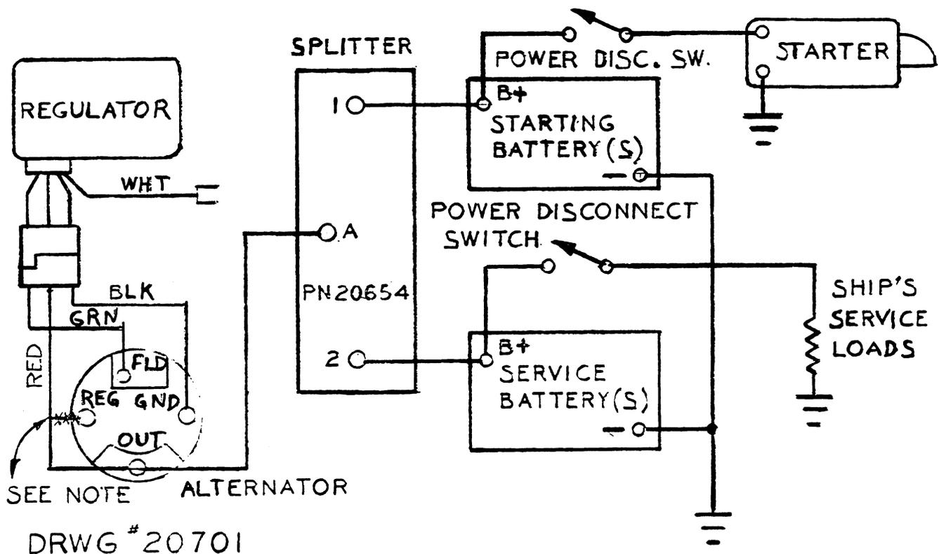
**NOTE:** On Alternators which have an isolation diode between their output and regulator terminals, such as the Motorola units used with most WESTERBEKE engines, the regulator wire should be removed from the REG terminal and reconnected to the OUTPUT terminal as shown. The diode in the splitter will provide an equivalent voltage drop.
